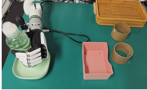
Figure 14: An example of the one-shot manipulation task. The robot picks up the bottle from the table, and infers the category of the object based on both visual input and tactile information, and finally places the object to the right place accordingly.
