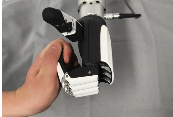
Figure 13: An example of the task CompliantControl. A person grabs the dexterous hand by applying external forces to a certain direction. The policy should infer the correct direction and move the end-effector according to tactility.
